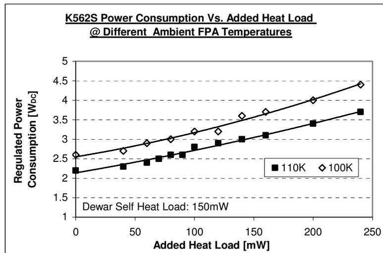
Figure 5: K562S Power Consumption Vs Added Heat Load at Different FPA Temp.
