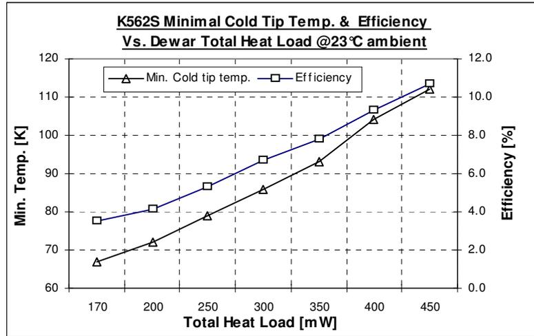
Figure 2: K562S Minimal Cold Tip Temp. & Efficiency Vs. Total Heat Load
