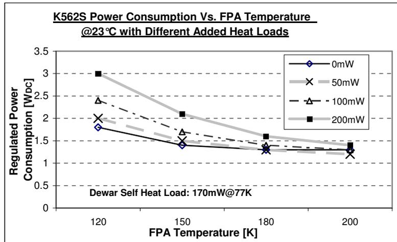
Figure 6: K562S Power Consumption Vs. FPA Temp. at Different Added Heat Loads
