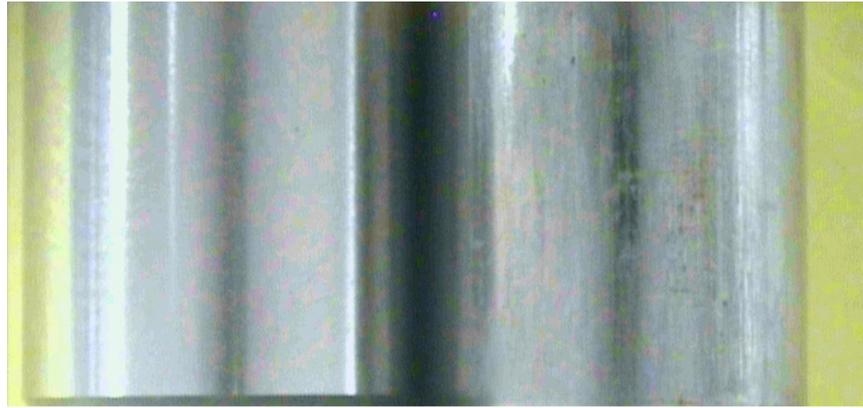
**Piston before** **Piston after 27,500 working hours**
