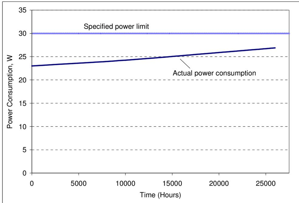
Figure 7: Stabilized power consumption vs. Time.
