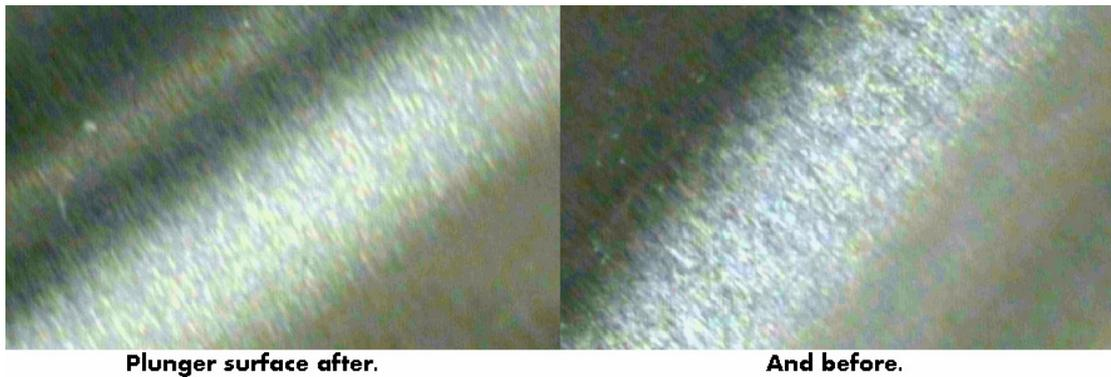
Figure 5: Plunger surface after and before 27,500 running hours.
