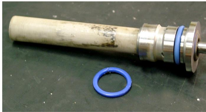
Figure 6: Cold head "after 27,500 working hours"
