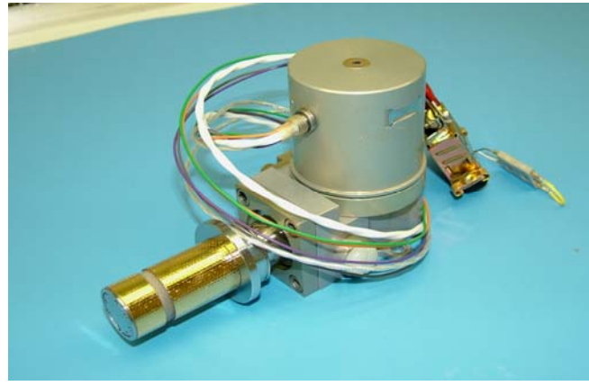
Figure 5. Coldfinger bumper attached to cooler.
