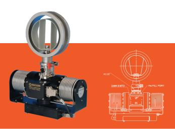
Based on the K535 cooler, the Cryo-Water Pump160 is an upgrade to an existing pump (mechanical or TMP) on load lock, transfer and/or process chambers. This combination provides high water vapor pumping speed, offering reduced partial pressure of water and total base pressure - together saving up to 50% of the pump down time.
