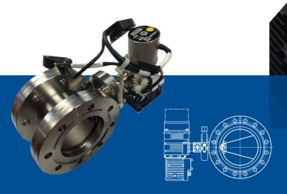
The Cryo-Water Pump100, Single Stage Cryopump, based on the K543 cryocooler, is the highest pumping speed member of the NanoStar\* line of cryopumps designed specifically for tabletop or small vacuum deposition tools, PVD / PEVD / CVD / ALD chambers, and load locks.
